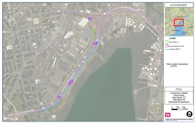
Figure 12. Alternative 3B, (Enhanced I-95 Embankment)
