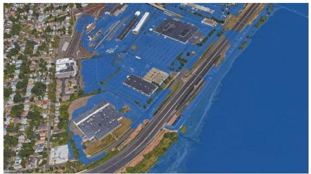
(Long Wharf, New Haven, CT focused study area: predicted flooding associated with the 2016 1% annual chance exceedance flood event. Flood simulations performed by GZA GeoEnvironmental, Inc., 2017)
