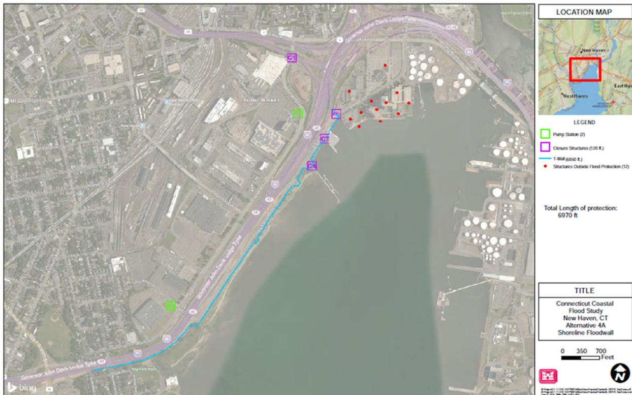
Figure E4: Alternative 4A Conceptual Design
