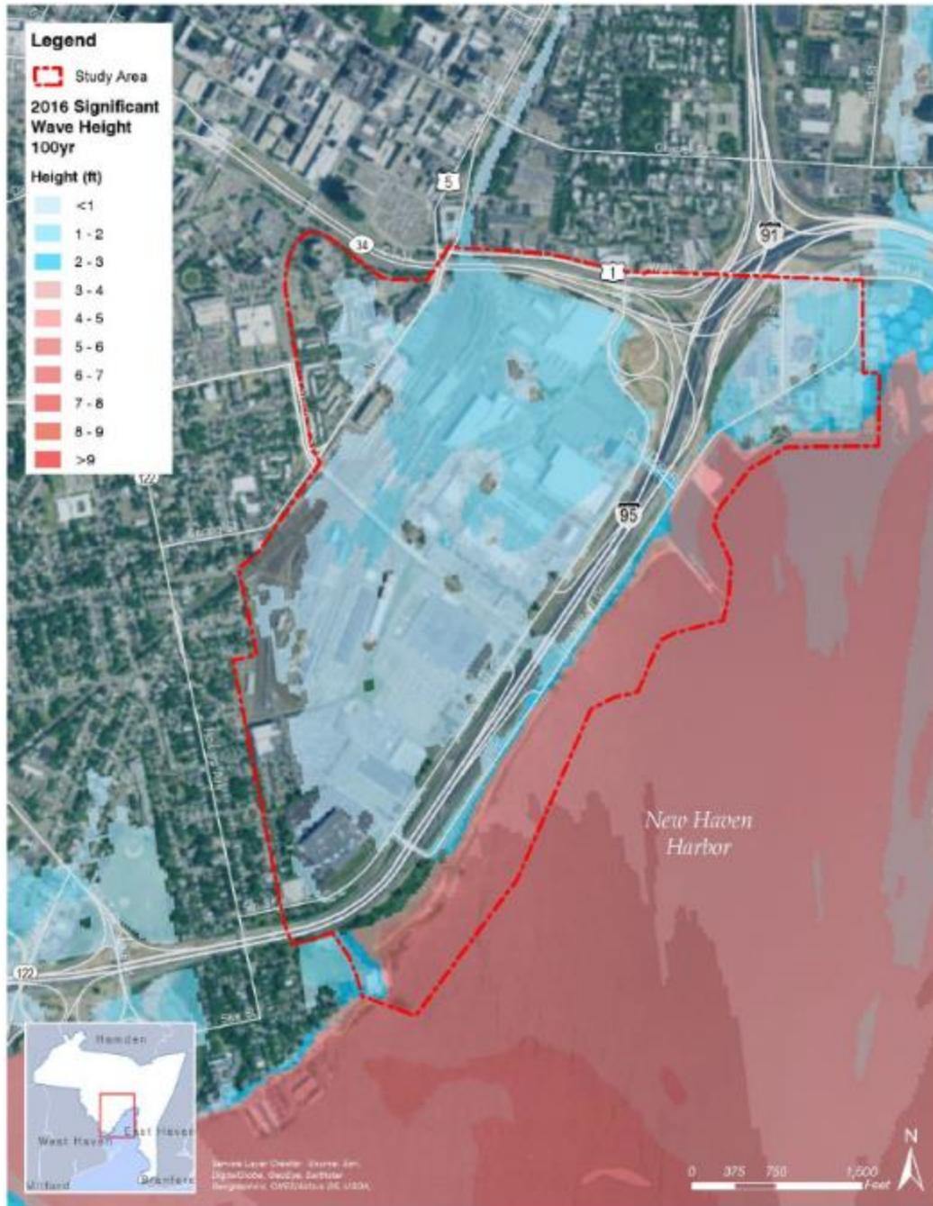
**Figure 3-9. Modeled significant wave height, in feet (GZA)**
