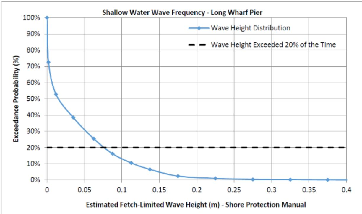
Figure 3-12. Nearshore wave frequency, Long Wharf Pier (GZA)
