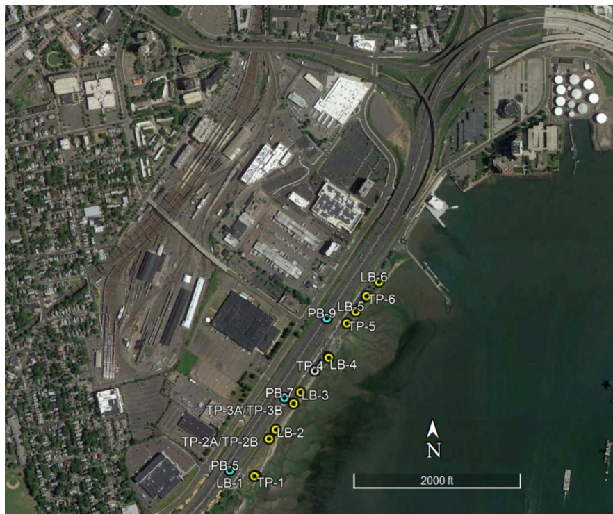
Figure 2: Location of borings utilized in design for New Haven
