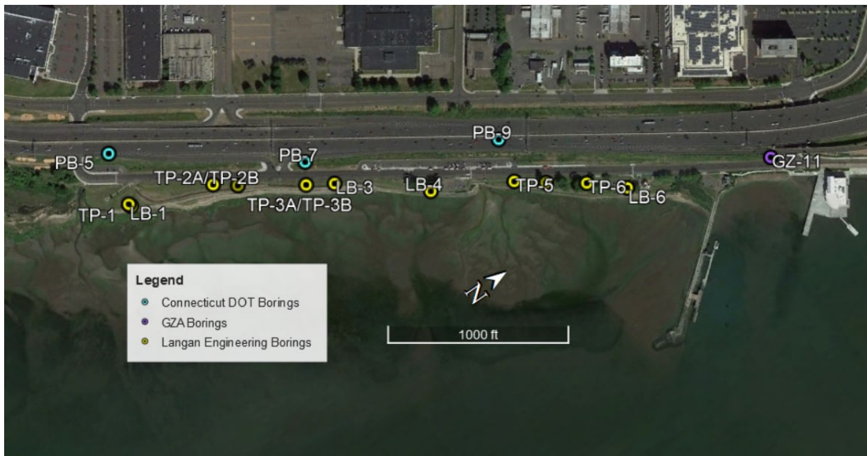
Figure 2.1: Location of borings utilized in design for New Haven
