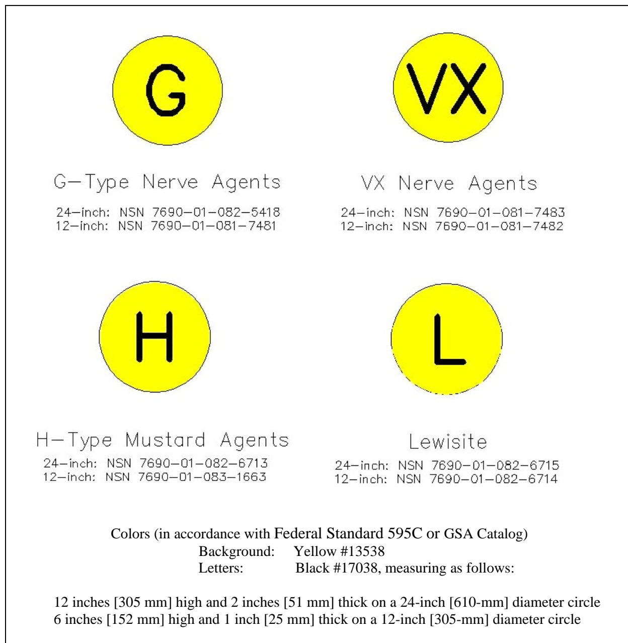
Figure V1.E10.F4. Supplemental Chemical Hazard Symbols
