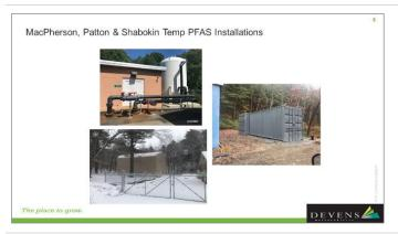
Jim Moore described the temporary WTP installations at MacPherson before it was insulated. He indicated that the Patton WTP is now waterproofed. The Shabokin WTP has four granular-activated carbon (GAC) filters in the insulated structure.
