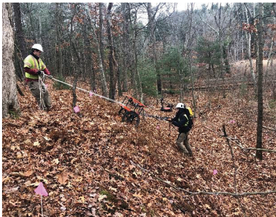
Photograph 1. Using EM61 in area AOC74. All AOI's were wooded. Pink flags represent the local grid set up for each area.
