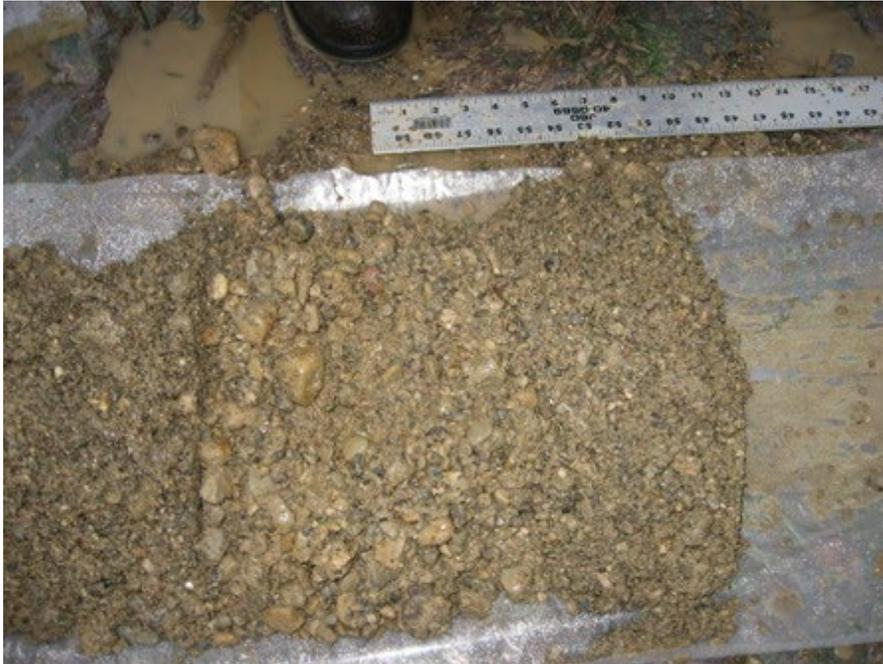
**10 -15 feet SAND, medium to very coarse, little granules to medium pebbles, subround to subangular, trace silt; poorly sorted, wet, grayish brown (10YR5/2).**
