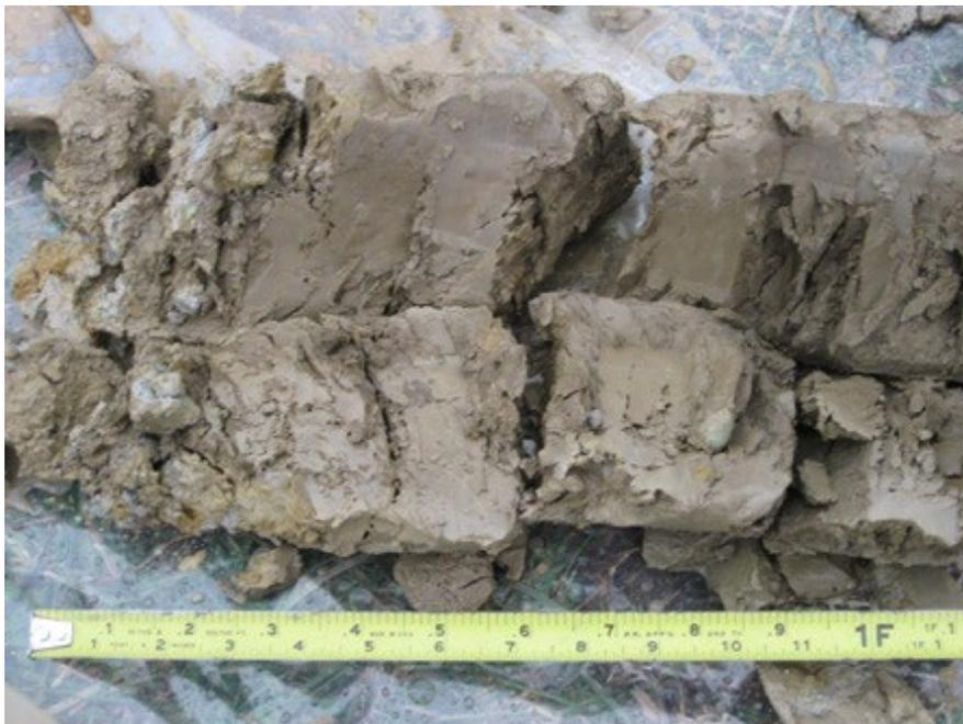
**10-15 feet CLAY, trace silt, trace small to very large pebbles, subround to subangular up to 2" diameter; medium to high plasticity, stiff, moist, dark grayish brown (10YR 4/2). NOTE: Lacustrine; laminated 0.1 to 0.2" thick, laminations brownish yellow (10YR 4/3).**
