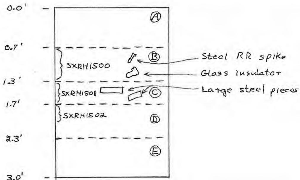
LAYER (A) - Sand, poorly graded, fine to coarse, mostly fine to med., <5% fines, ~10% coal dust, fibrous roots, humic material, loose, dry, dark olive brown (2.5Y/3/3), SP. Cobbles to 3".
