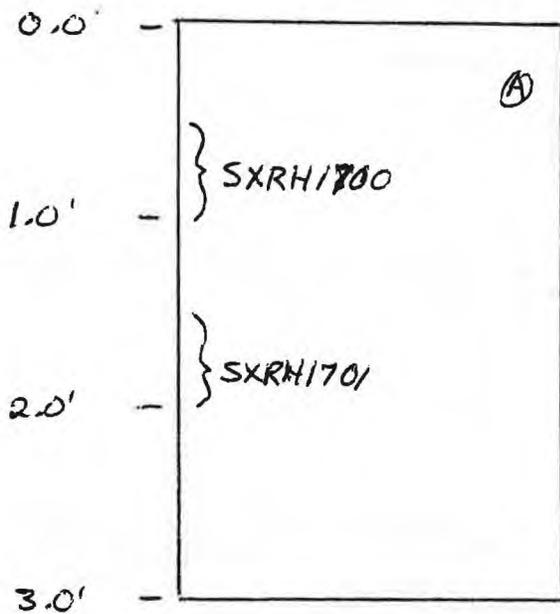
LAYER (A) - Gravelly sand, well graded, cobbles to 6" max., coarse to fine sand, 10-15% fine gravel, < 5% fines, loose to medium dense, moist, very pale brown (10YR/7/3) SW
