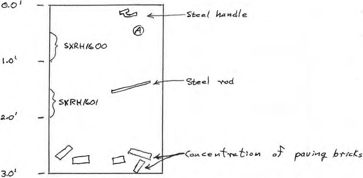
LAYER **A** - Coal ash, coal, and clinker, from dust-size grains to cobble-size clinker, some fine sand (<20%) in upper 1 foot, dense, dry, dark gray (SX/4/1)
