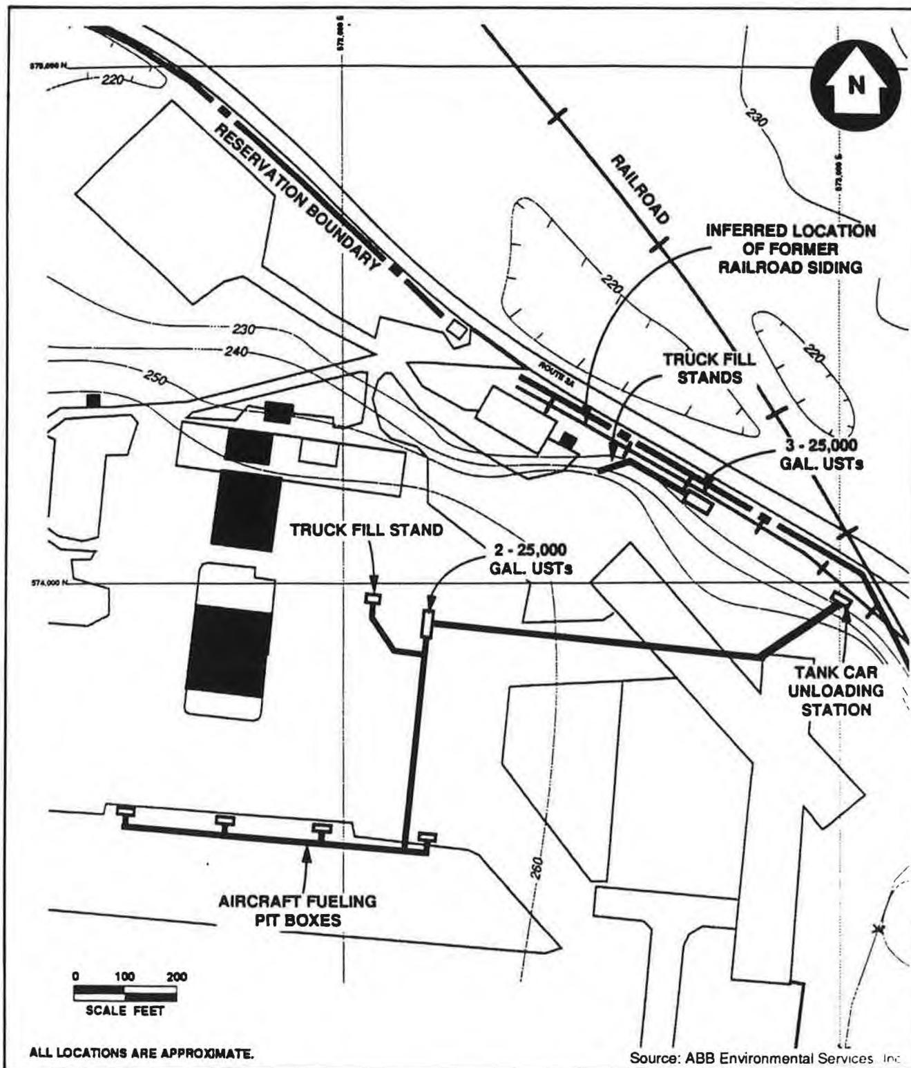
**FIGURE 3-5 APPROXIMATE LOCATION OF FEATURES ASSOCIATED WITH WWII FUEL POINTS (AREA 50)**
