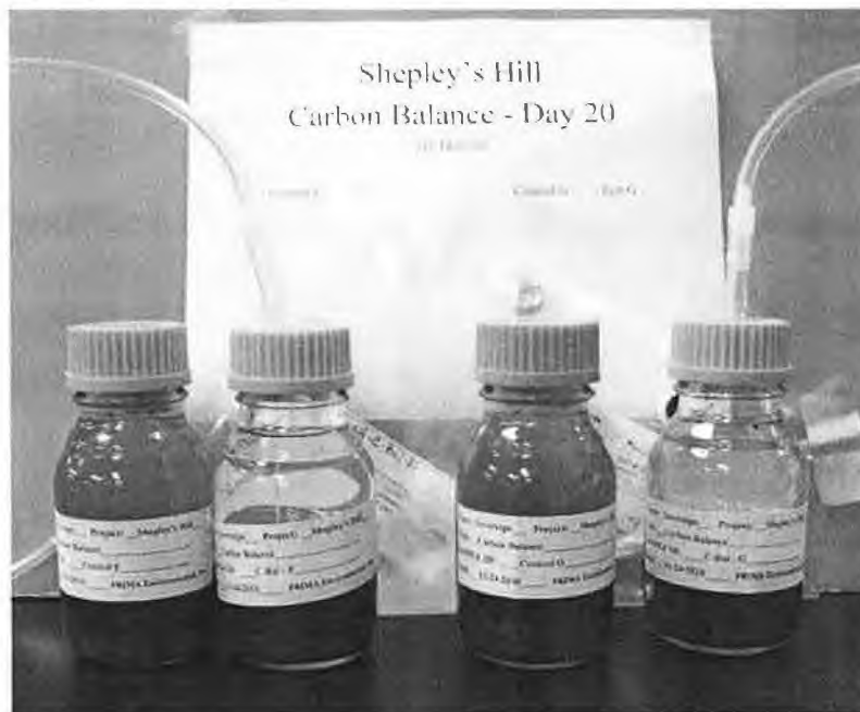
Figure 4. Example Carbon Balance Reactors at Day 20. Non-sterilized (no added azide) reactors are connected to Tedlar bags.
