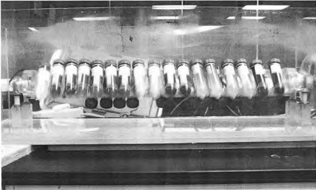
Figure 3. Sequential Extraction Apparatus – end-over end rotator.
