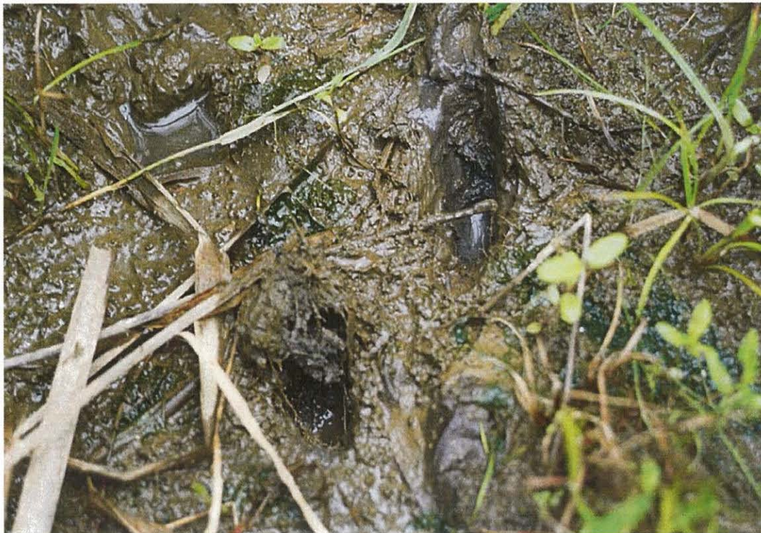
AOC 57 Area 2: Close-up of a finger scoop of wetland sediment showing the underlying hydric soil (darker color) covered by a layer of fine silt (lighter brown color) as a result of erosion from
