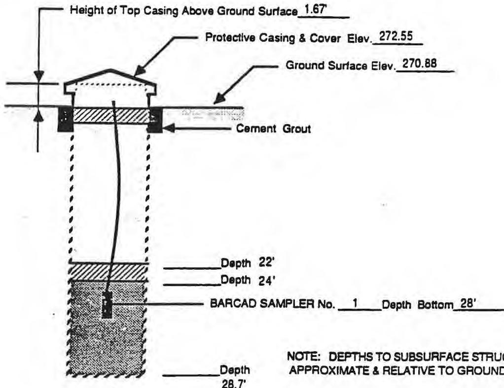
MONITORING WELL CROSS-SECTION WITH BARCAD SAMPLER INSTALLATION
