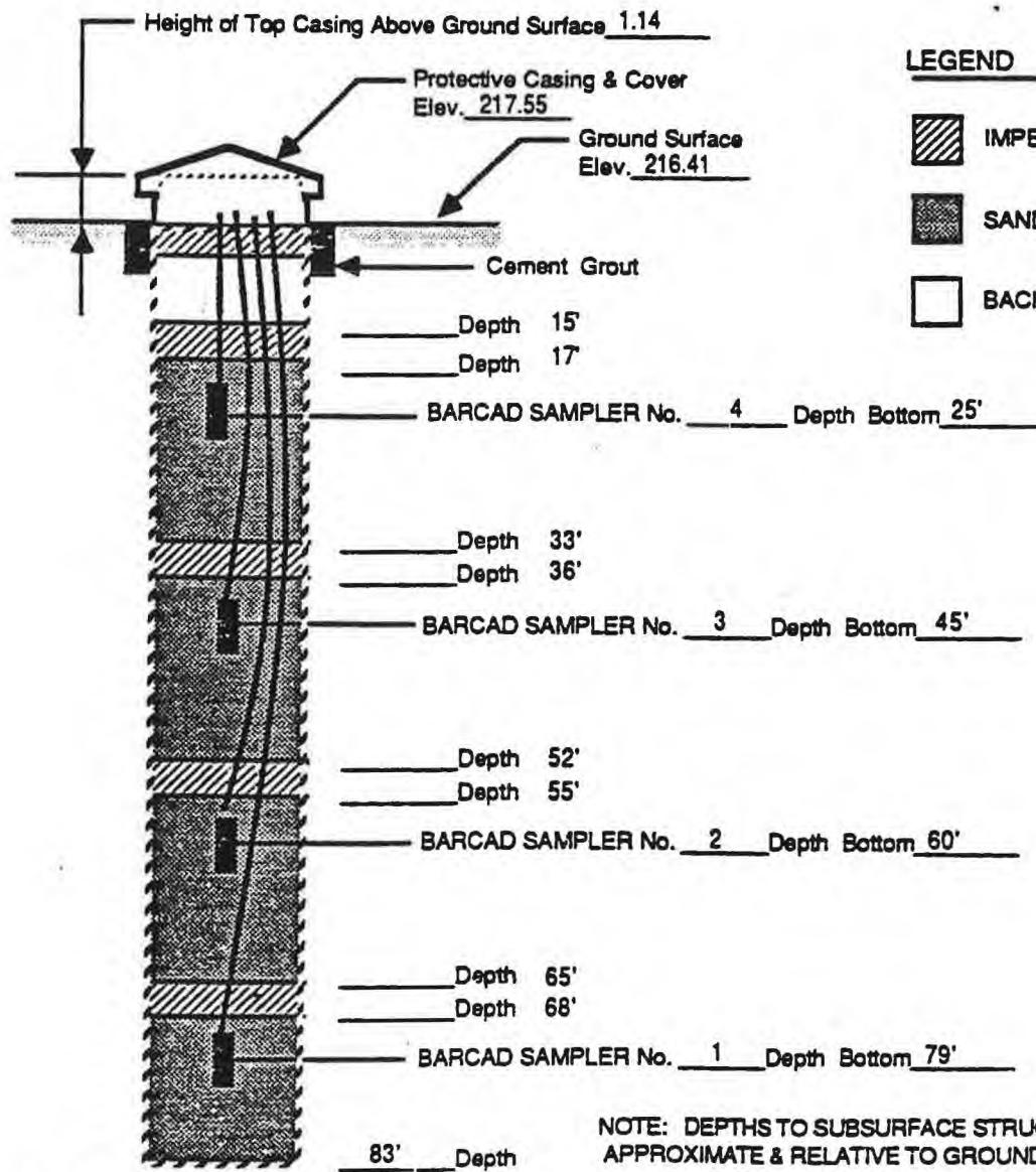
MONITORING WELL CROSS-SECTION WITH BARCAD SAMPLER INSTALLATION
