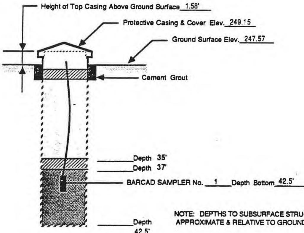
**MONITORING WELL CROSS-SECTION WITH BARCAD SAMPLER INSTALLATION**
