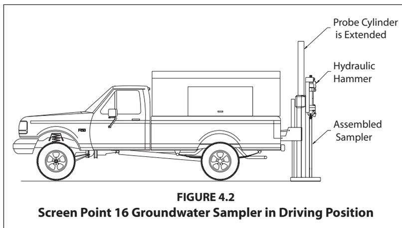
4. Repeat Step 3 until the desired sampling interval is reached. Approximately 12 inches (305 mm) of the last probe rod must extend above the ground surface to allow attachment of the puller assembly. A 12-inch (305 mm) rod may be added if the tool string is over-driven.
