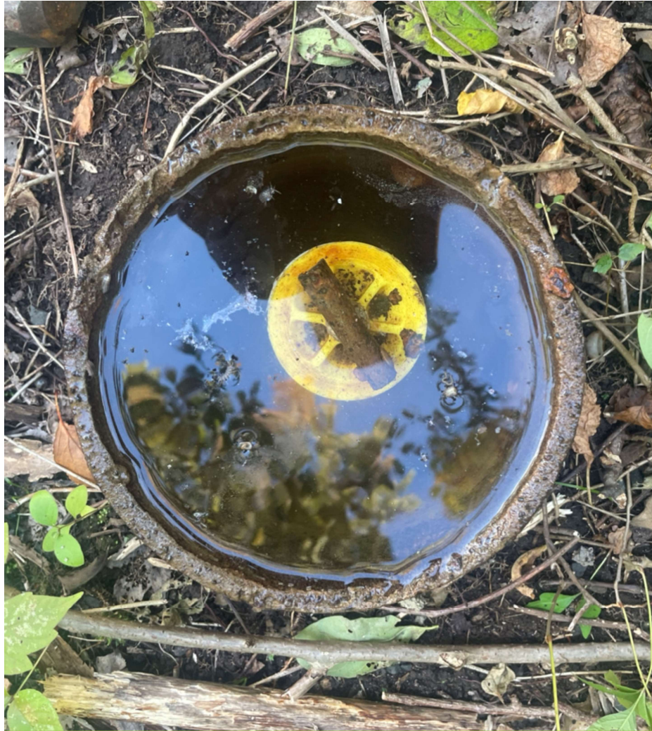
Picture 1: Well MMC-MW-6, which was previously converted to a 2" PVC monitoring well.
