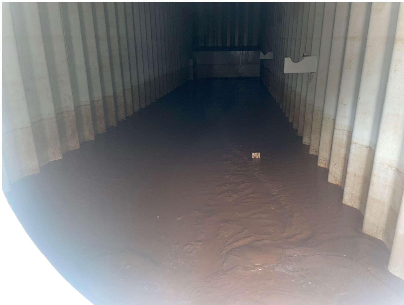
Picture 4: Silt remaining in the frak tank after Ludlow pumped stored groundwater through a treatment system staged at the 281 Main Street, Durham work yard.
