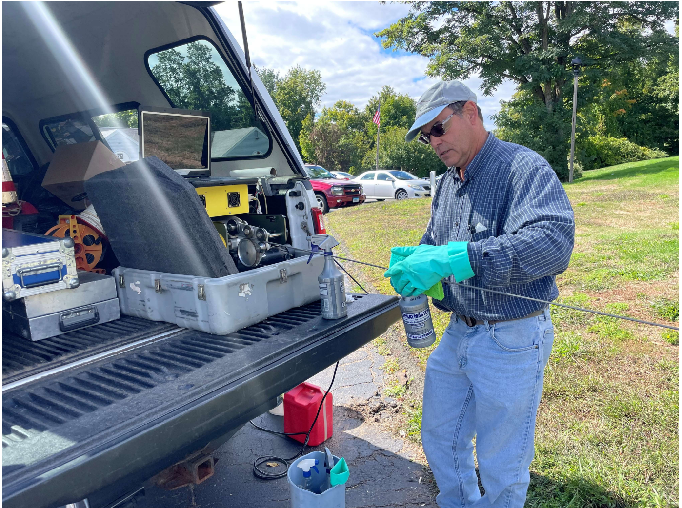
Picture 7: Geophysical Applications decontaminating the cable used to lower probes into the well located at the Hill Hollow condominium complex in Durham.
