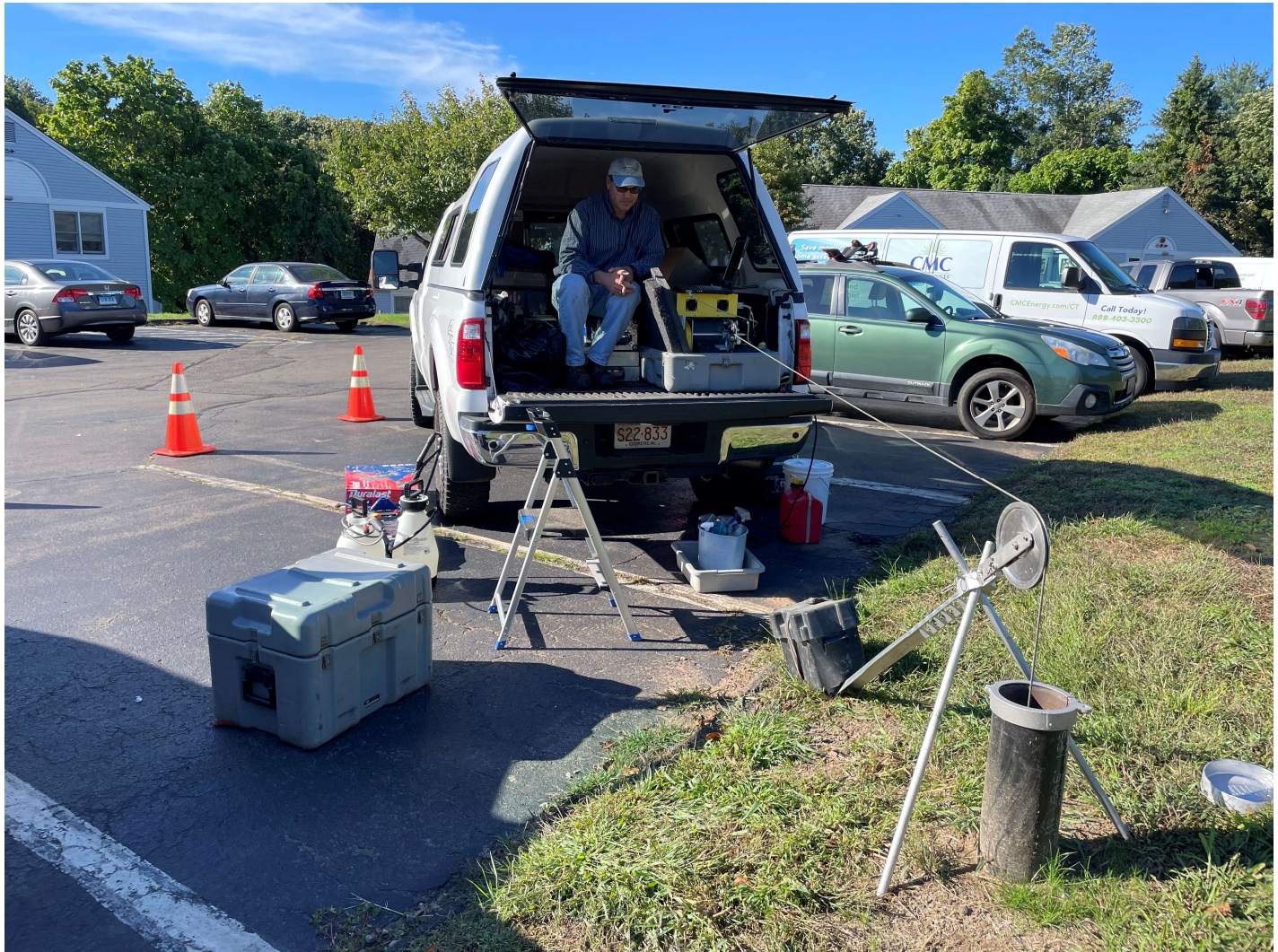
Picture 3: Geophysical Applications performing borehole assessment activities on the well located at the Hill Hollow condominium complex in Durham. View to the southwest.
