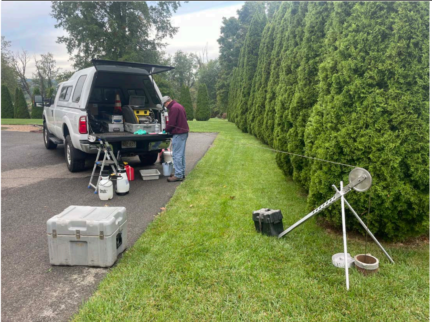
Picture 1: Geophysical Applications set up to perform borehole assessment activities on the well located on the north side of the 166 Maple Avenue, Durham, residence. View to the west.
