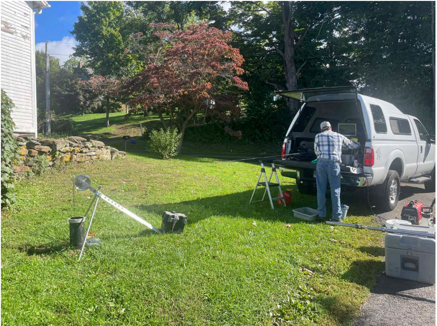
Picture 3: Geophysical Applications set up to perform borehole assessment activities on the well located on the south side of the 110 Maple Avenue, Durham, residence. View to the northeast.
