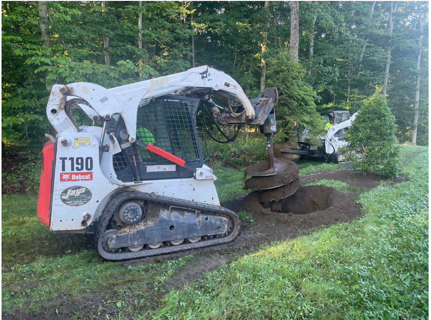
Picture 1: Jays Landscaping auguring a hole as they prepare to plant one of the 19 trees scheduled to be placed on the south side of the water tank located to the east of the Shared Access Driveway in Middletown. View to the west.
