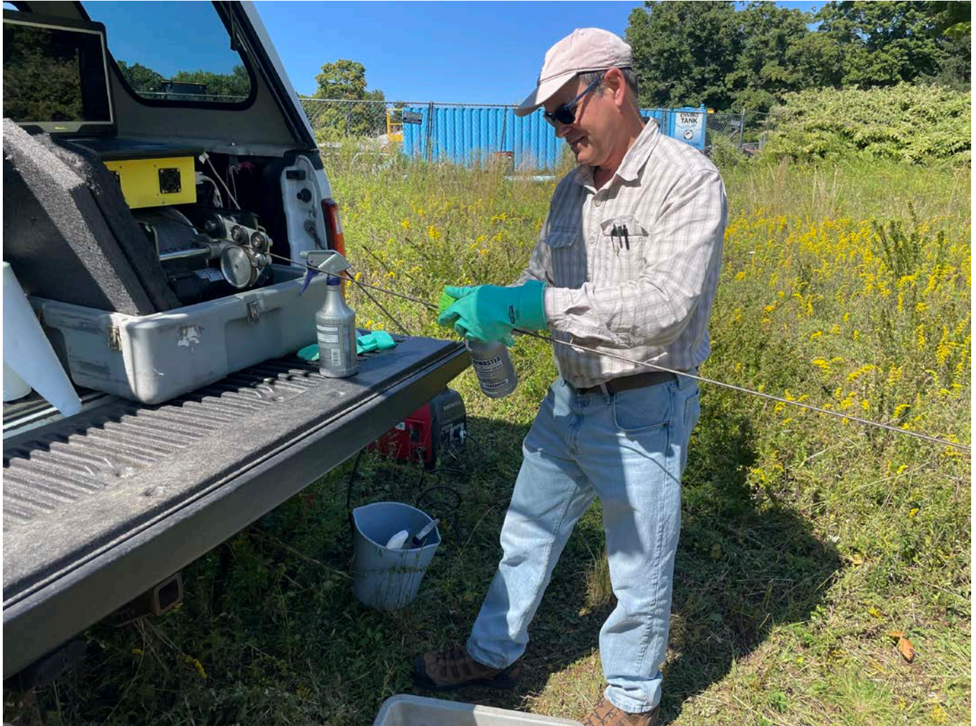
Picture 7: Geophysical Applications decontaminating a section of cable that is being used to lower borehole assessment instruments into well number MW-2, which is located on the east side of the 281 Main Street, Durham, property.
