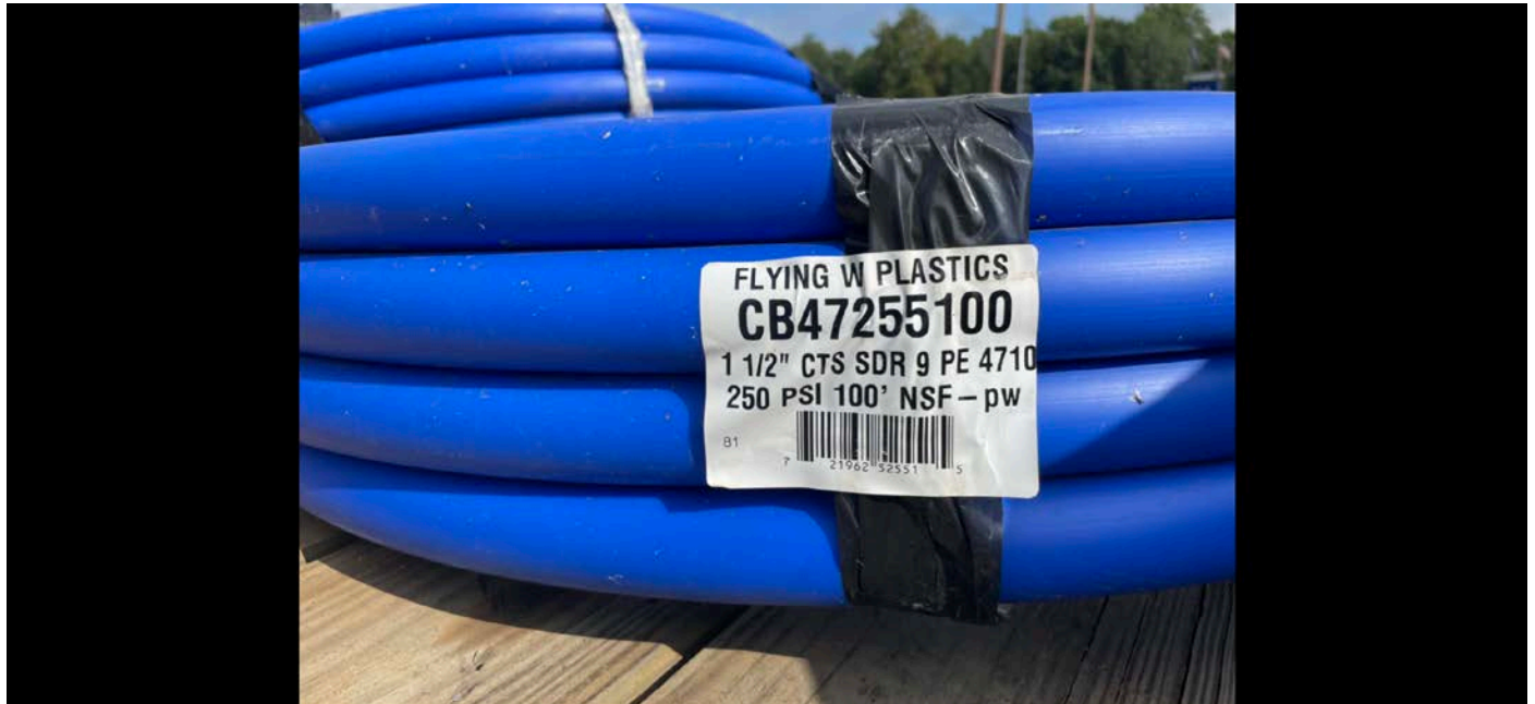
Picture 4: 1.5" polyethylene water line that Ludlow installed between the recreation center and the meter vaults located at Station ~516+55.
