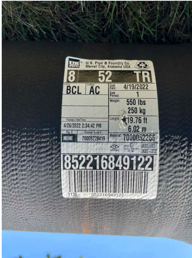
Picture 3: A section of 8" DIP that Ludlow is installing at Station 529+64 on Pickett Lane, Durham.
