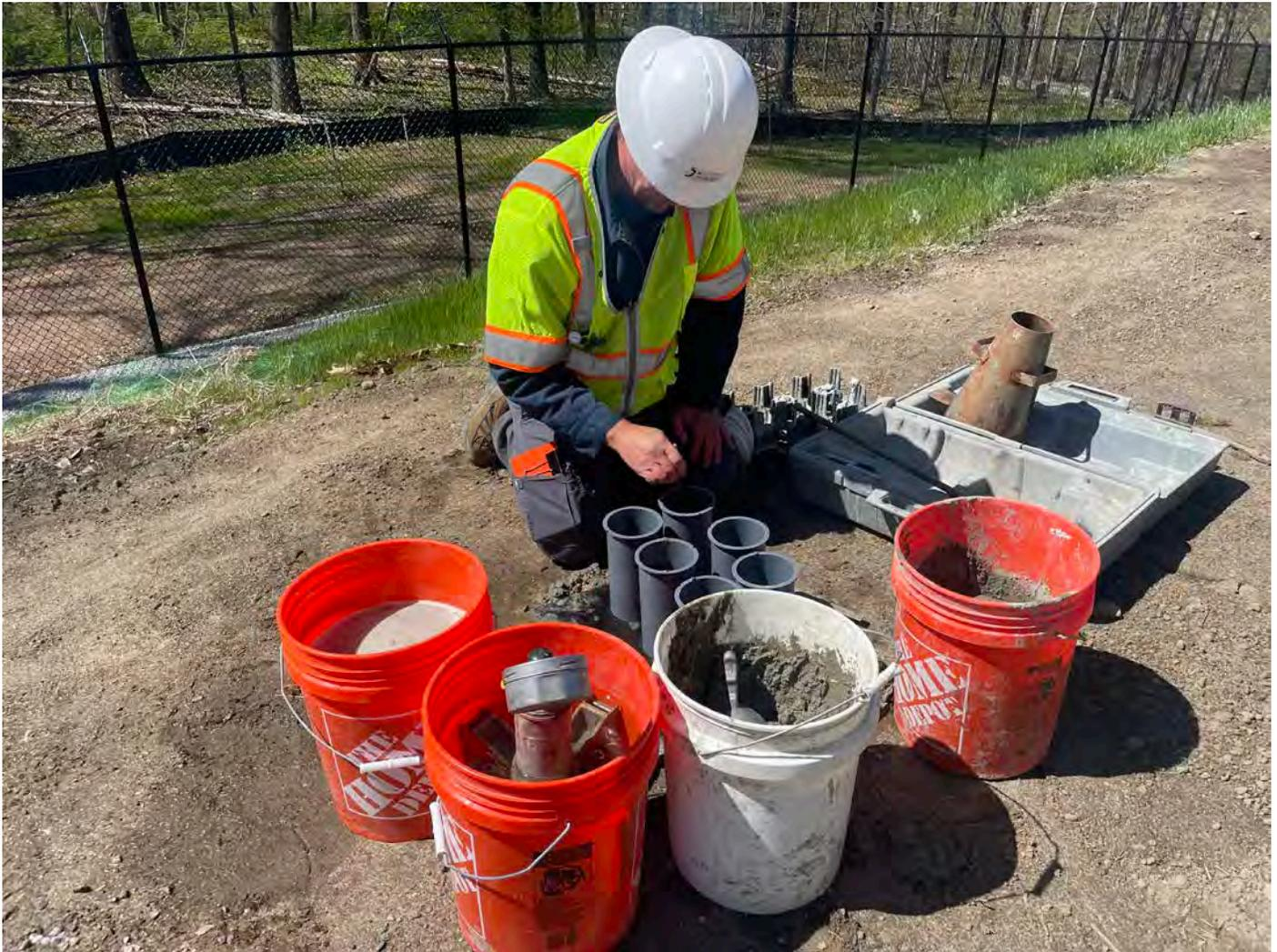
**Picture 6: JTC preparing QC samples collected from the first load of 4000 PSI mix that Farmington Ready-Mix delivered to the water tank work zone. View to the southwest.**
