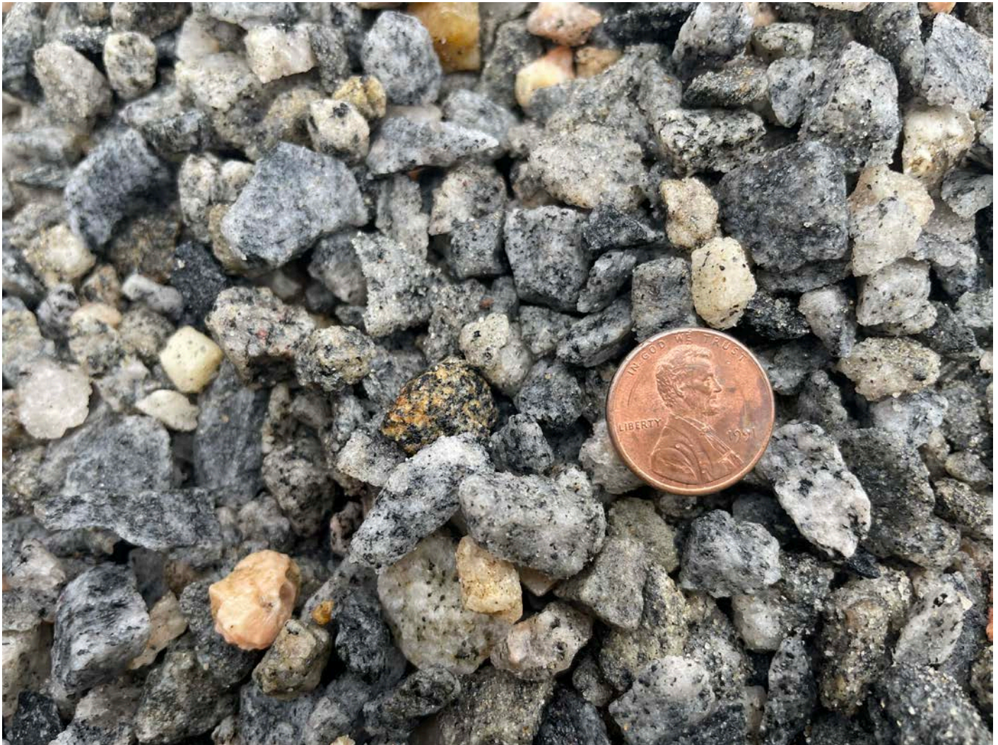
Picture 13: Closeup of the 3/8" stone that Ludlow is placing over black geofabric along the bottom of the fence that surrounds the water tank located east of the Shared Access Driveway in Middletown.
