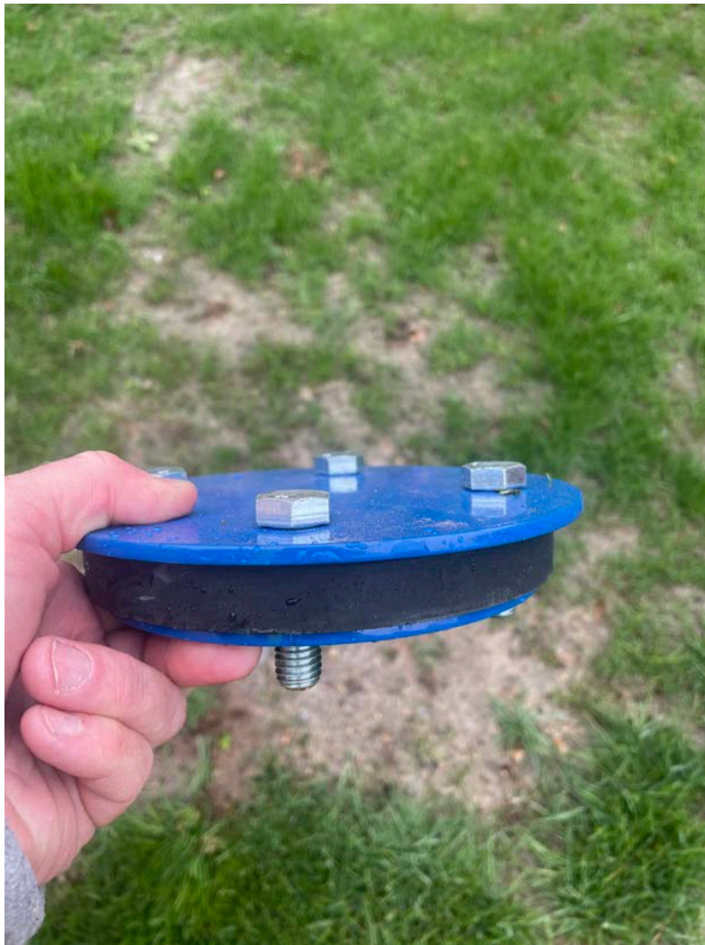
Picture 9: Expanding well cap that Grela has been placing on top of the well casing after removing a pump from a well.
