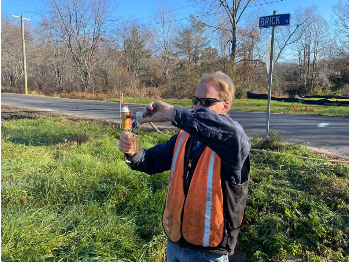
Picture 3: JMS testing for residual chlorine during the dechlorination process. View to the northeast.
