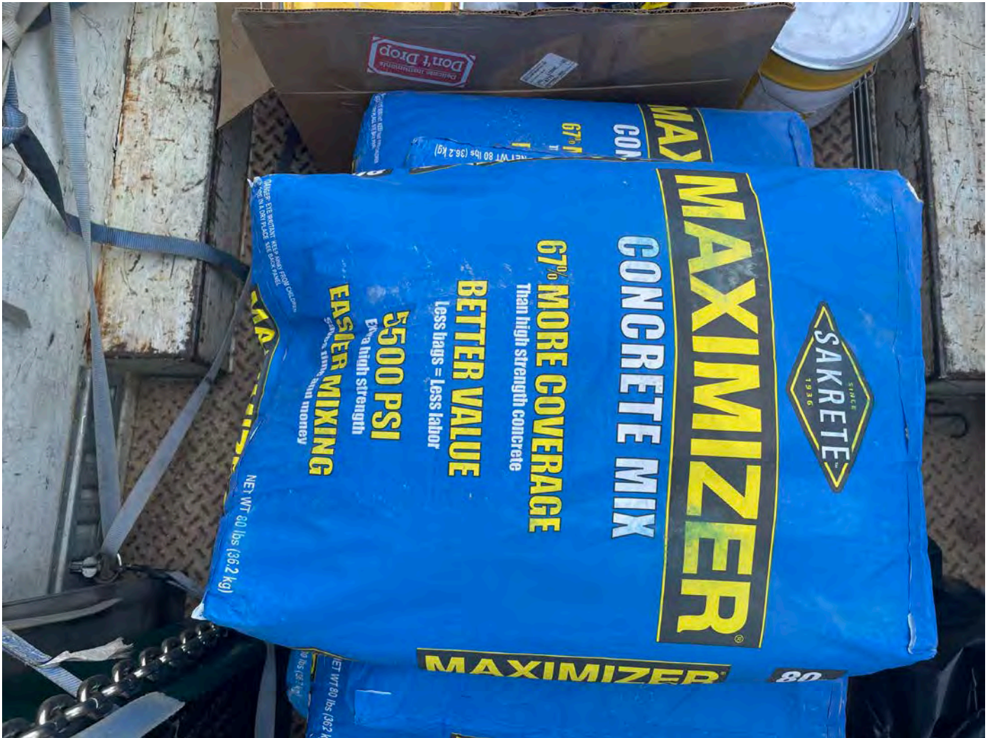
Picture 7: 5500 PSI concrete mix that United Concrete used to fill cut-outs in the water meter building floor.
