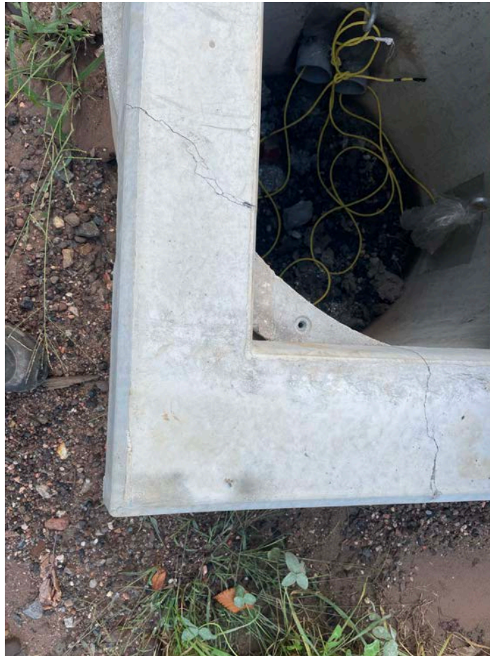
Picture 3: Damaged transformer slab at Station ~11+50 that Ludlow returned to United Concrete today.
