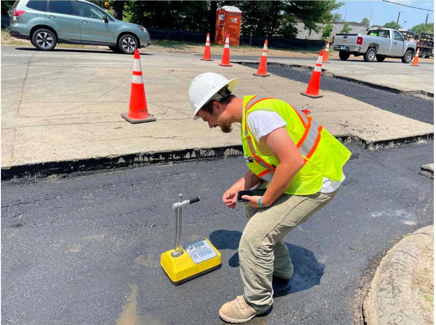
Picture 8: JTC testing compaction on the first lift of asphalt that was placed on the trench overcuts on the northbound lane of S. Main Street, Middletown. View to the west.
