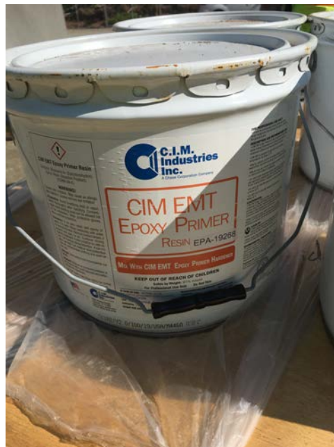
Picture 2: Epoxy primer for sealing seams on the inside of the tank.
