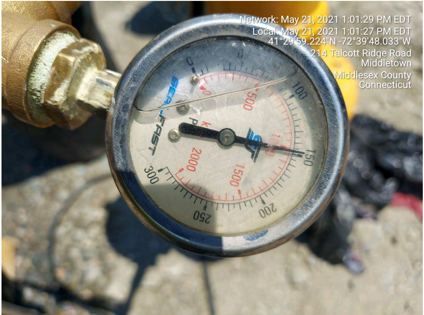
Picture 11: End pressure on the pressure test that Ludlow is running from the water tank located east of the Shared Access Driveway to a valve located on the Talcott Ridge Drive cul-de-sac.
