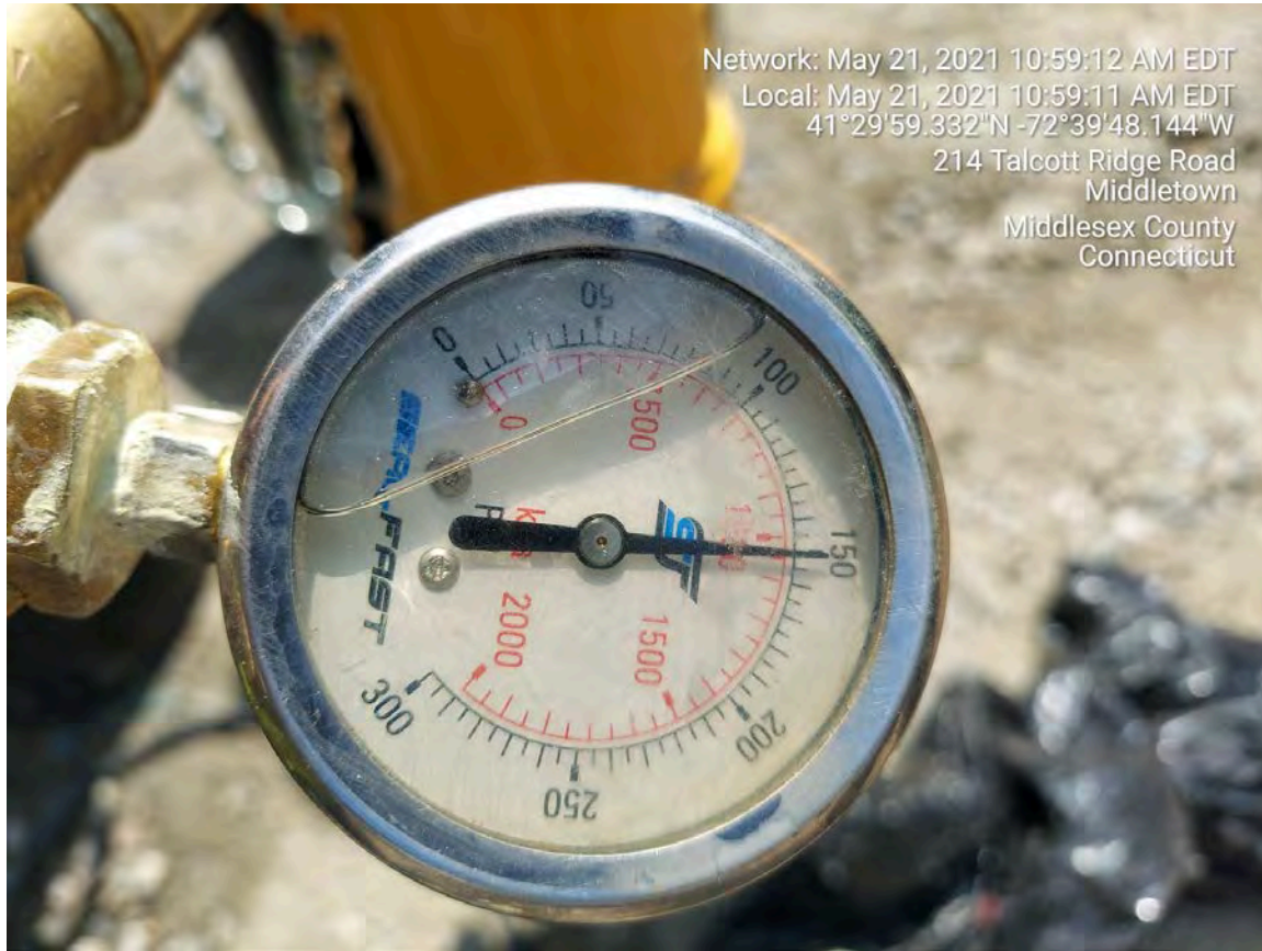
Picture 7: Starting pressure on the pressure test that Ludlow is running from the water tank located east of the Shared Access Driveway to a valve located on the Talcott Ridge Drive cul-de-sac.
