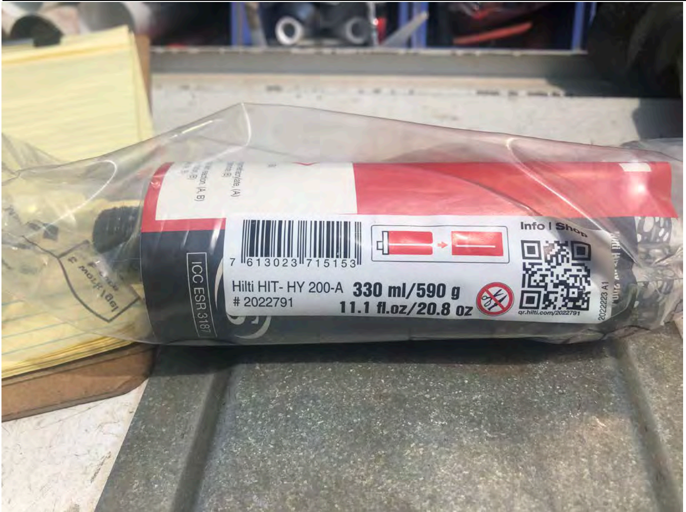
Picture 5: Hilti – HIT HY 200-A injectable hybrid mortar that United concrete is using to cover holes where segments of rebar penetrate the booster station floor and go into the top of the frost wall.
