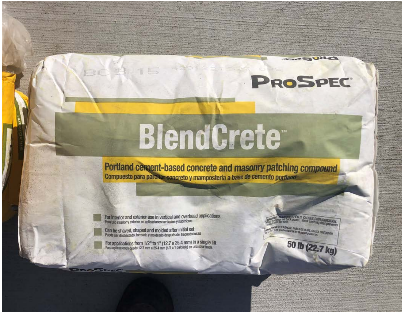
Picture 3: Grout that United Concrete will use on the bottom sections of the altitude valve vault. East of the Shared Access Driveway, Middletown.
