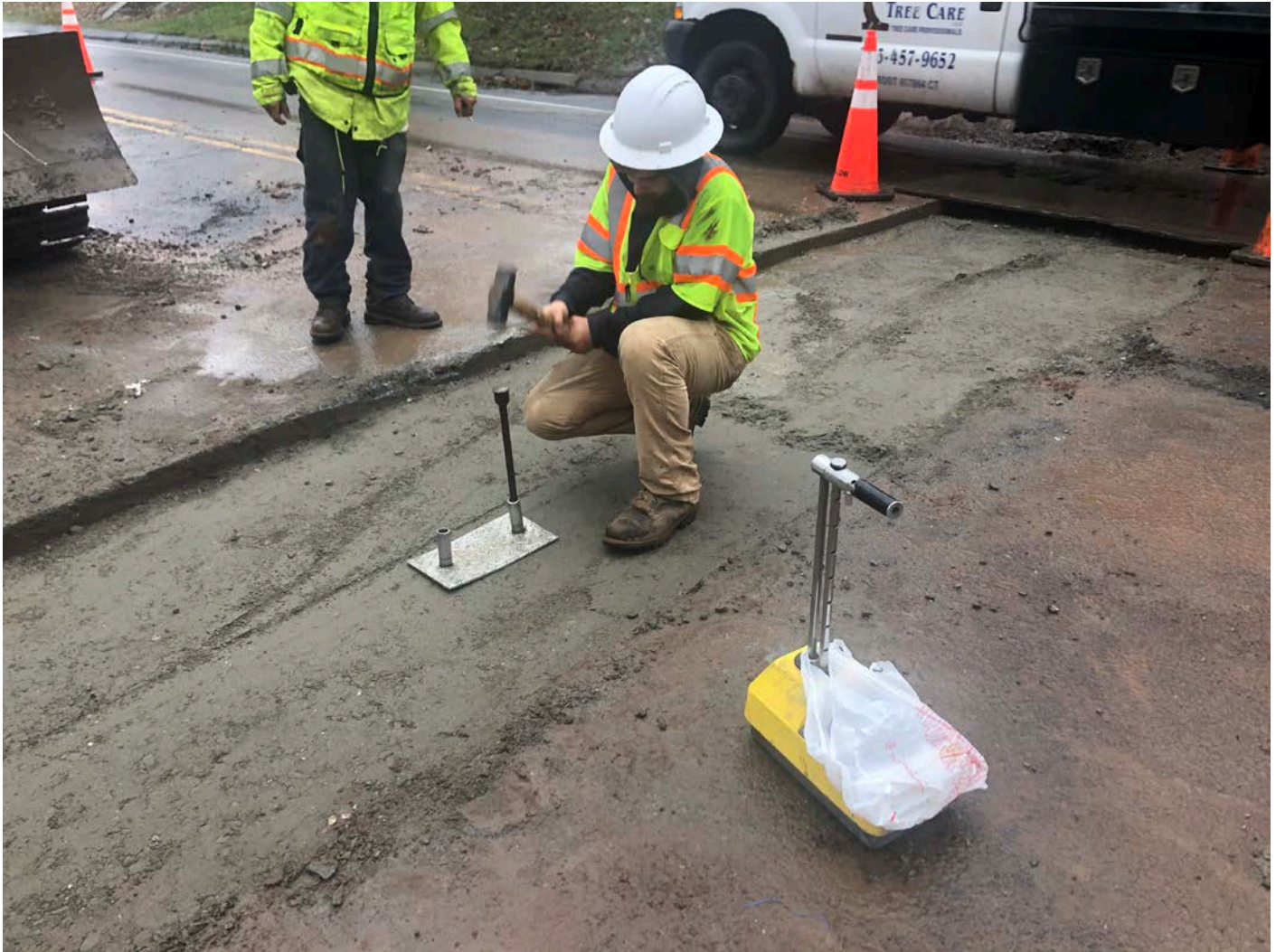
Picture 10: JTC collecting compaction data from the compacted soils in the trench that Ludlow excavated for the installation of a water service at 119 Main Street, Durham.
