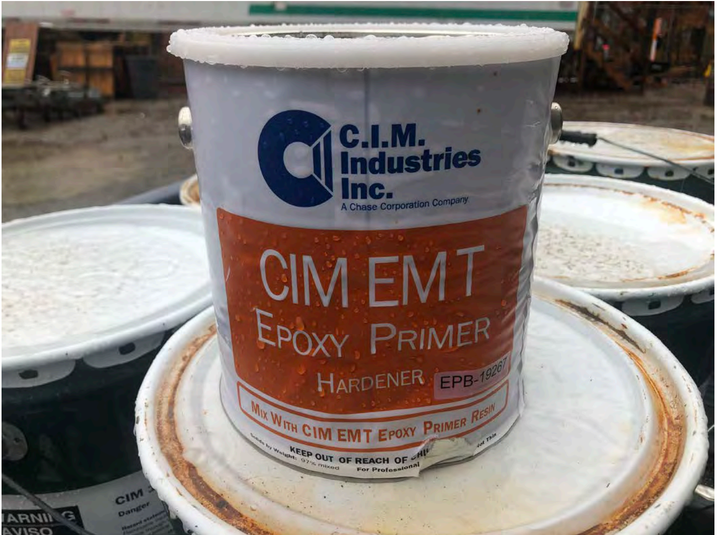
Picture 4: Part two of the two-part coating that will be applied to the interior of the water tank. Water tank work zone located to the east of the Shared Access Driveway, Middletown.
