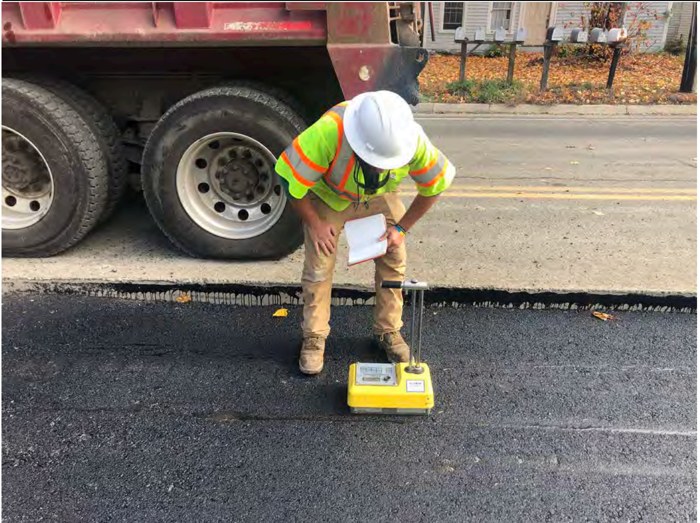
Picture 5: JTC collecting compaction data from the first lift of asphalt that Ludlow placed and compacted between Stations 192+70 and 195+30 on the southbound lane of Main Street, Durham. View to the east.
