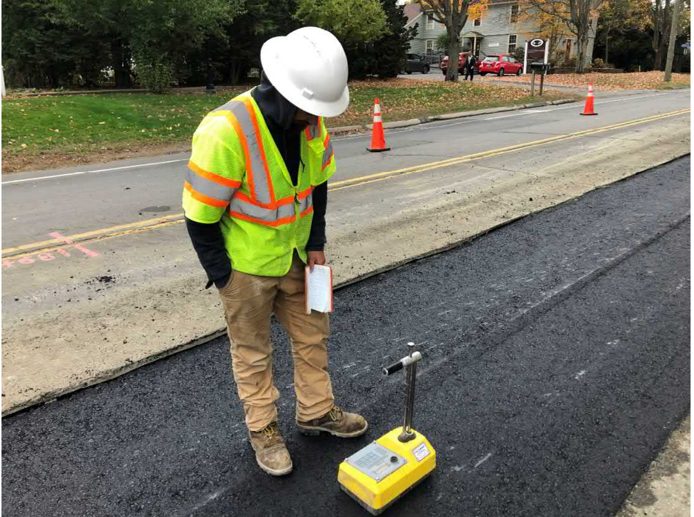
Picture 5: JTC collecting compaction data from the second lift of asphalt that Ludlow placed and compacted between Stations 189+00 and 192+70 on the southbound lane of Main Street, Durham. View to the southeast.
