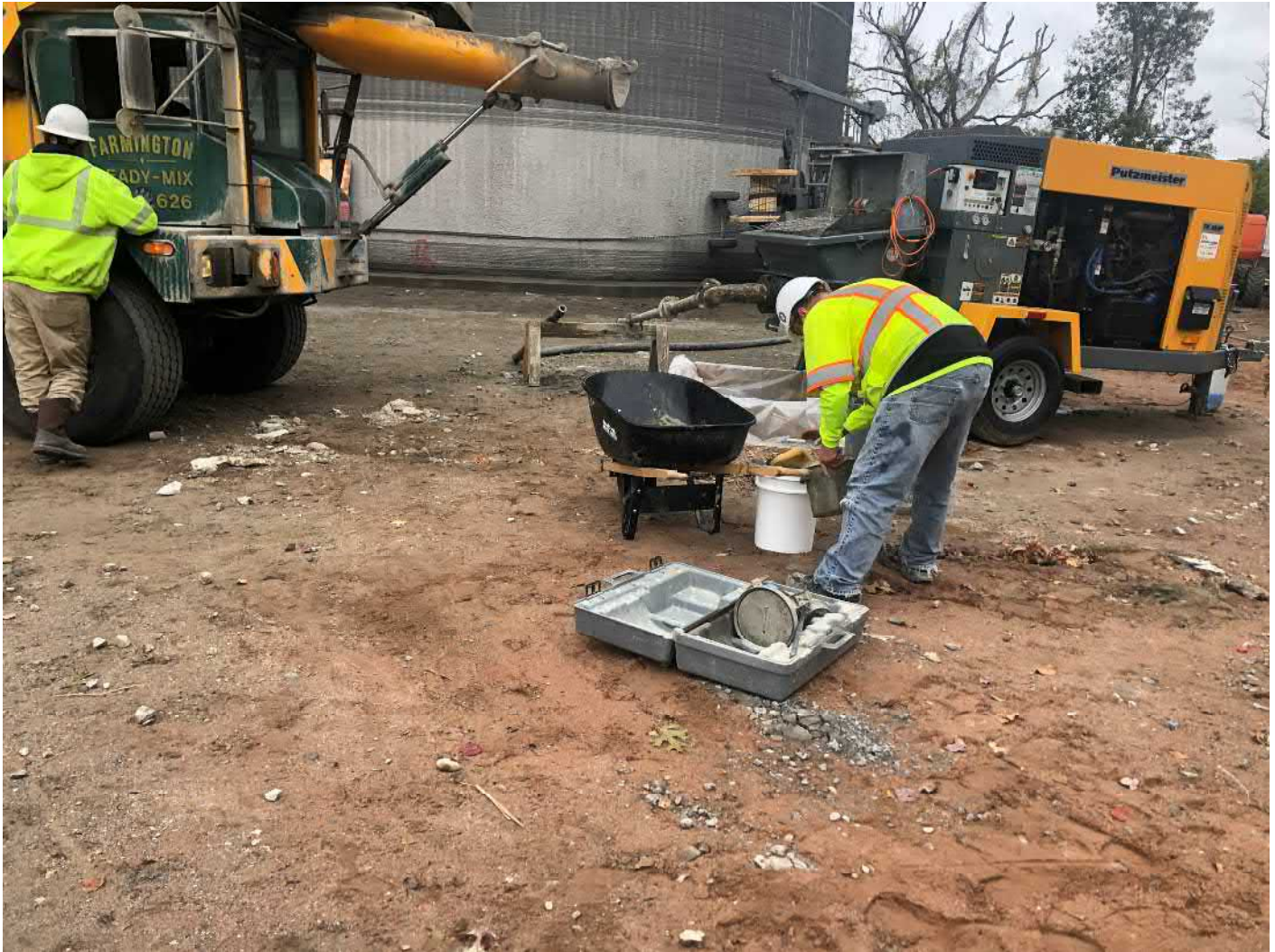
Picture 9: JTC preparing an air entrainment sample from a truckload of shotcrete that DN Tanks is about to apply to exposed prestressed wire on the exterior of the water. Water tank work zone located to the east of the Shared Access Driveway, Middletown.
