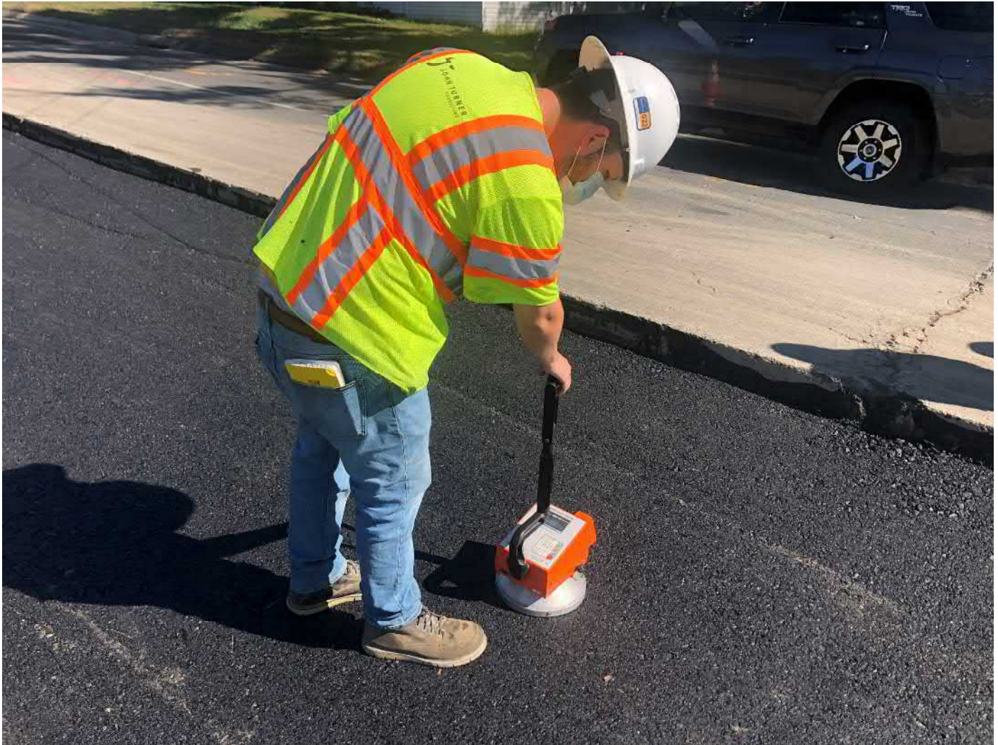
Picture 5: JTC collecting compaction data from permanent paving at trench cutbacks between Stations 160+25 and 163+55 on the southbound lane of Main Street, Durham. View to the northeast.
