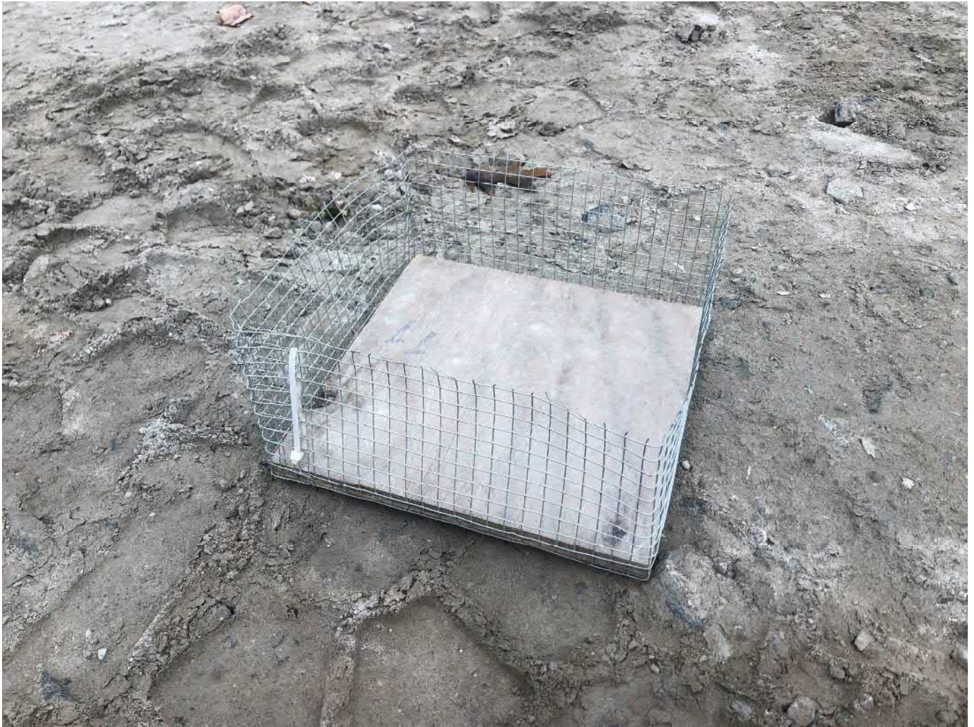
Picture 3: Basket used for the collection of a sample of shotcrete. Water tank work zone, east of the Shared Access Driveway, Middletown.
