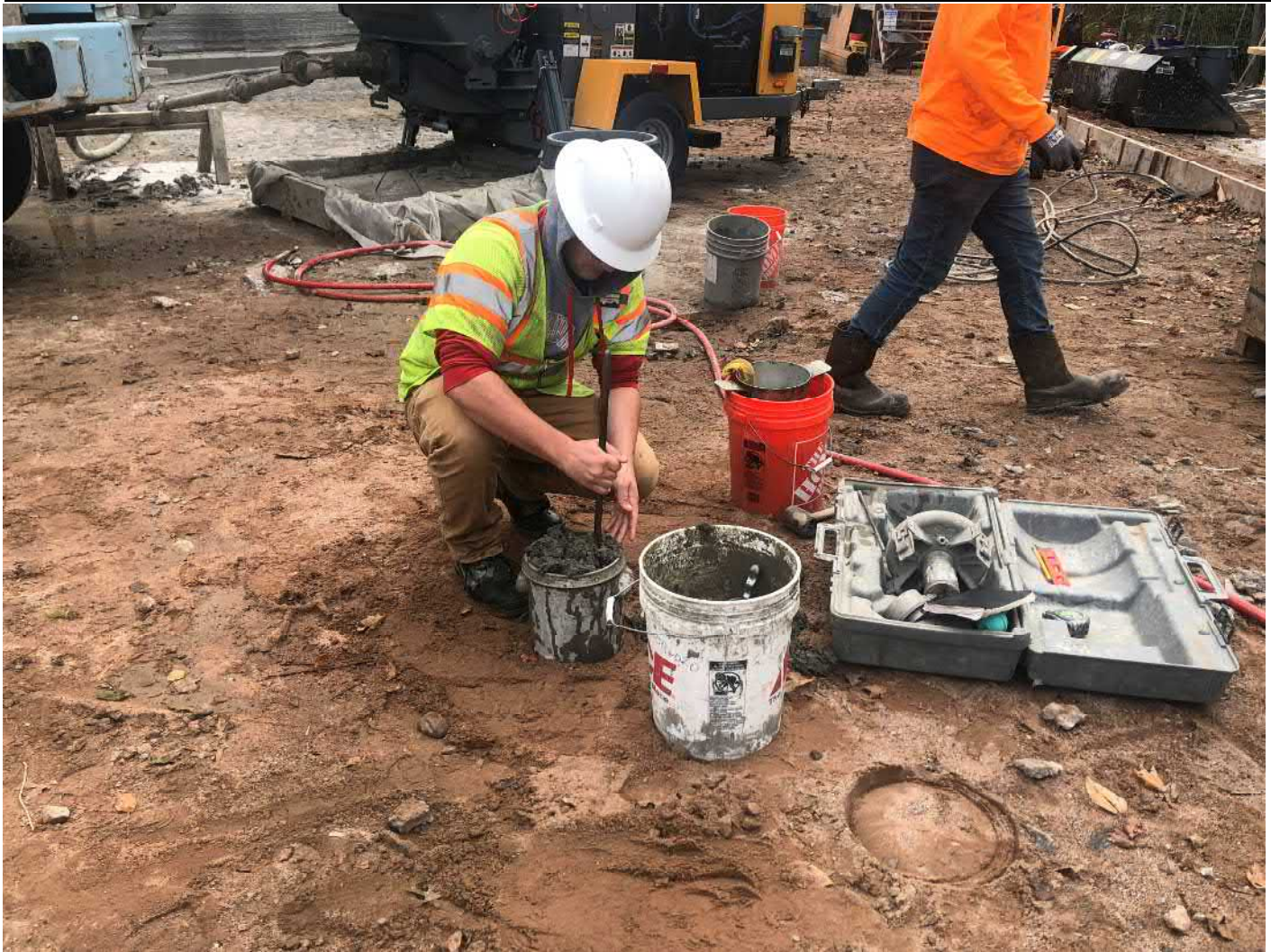
Picture 5: JTC preparing an air entrainment sample from the first of three trucks of shotcrete delivered to the water tank work zone located to the east of the Shared Access Driveway, Middletown. View to the east.
