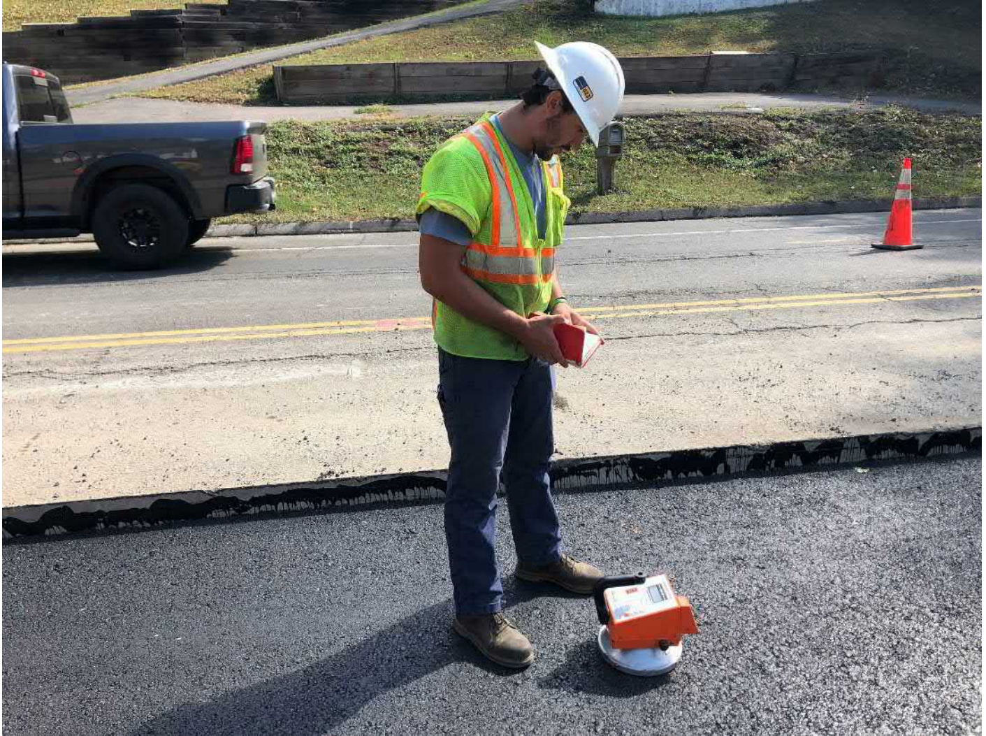
Picture 7: JTC collecting compaction data from the first of three 3" lifts of asphalt on the southbound lane of Main Street, Durham from Stations 143+00 to 146+30. View to the southeast.
