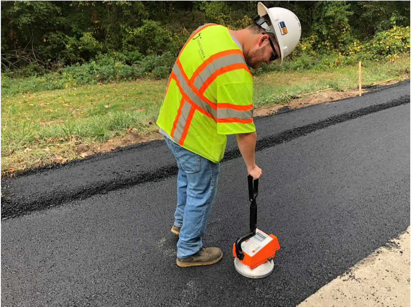
Picture 8: JTC collecting compaction data from asphalt placed between Stations 136+95 and 140+50 on the southbound lane of Main Street, Durham. View to the northwest.
