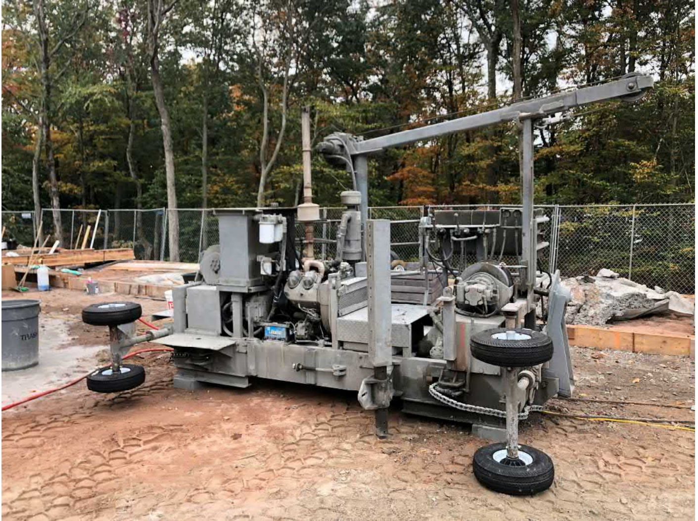
Picture 2: Machine that DN Tanks will use to start the placement of prestressed wire around the shotcrete that was placed on the exterior of the water tank yesterday. Water tank work zone, east of the Shared Access Driveway, Middletown. View to the south.
