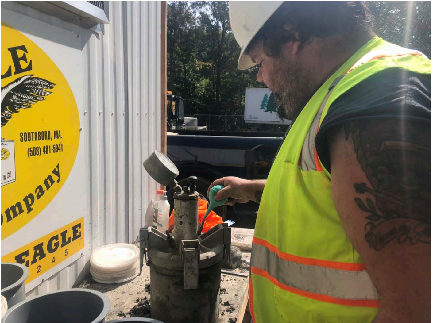
Picture 5: JTC performing air entrainment test on concrete brought to the site to be placed on top of the water tank today. Water tank work zone east of the Shared Access Driveway, Middletown.
