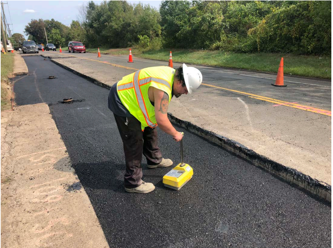
Picture 9: JTC collecting compaction data from the top of compacted asphalt on S. Main Street, Middletown as part of trench cutback repaving activities. View to the northwest.
