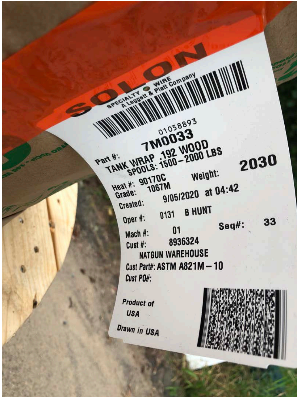
Picture 3: Tag attached to the prestressed wire that was delivered to the water tank work zone, east of the Shared Access Driveway, Middletown.
