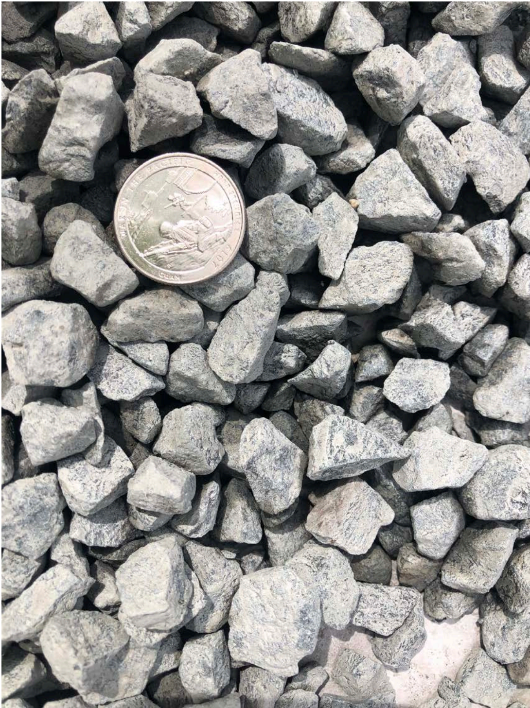
Picture 5: Stone placed around the 6" underdrain pipe placed by Ludlow around the periphery of the water tank base. Water tank work zone, east of the Shared Access Driveway, Middletown.
