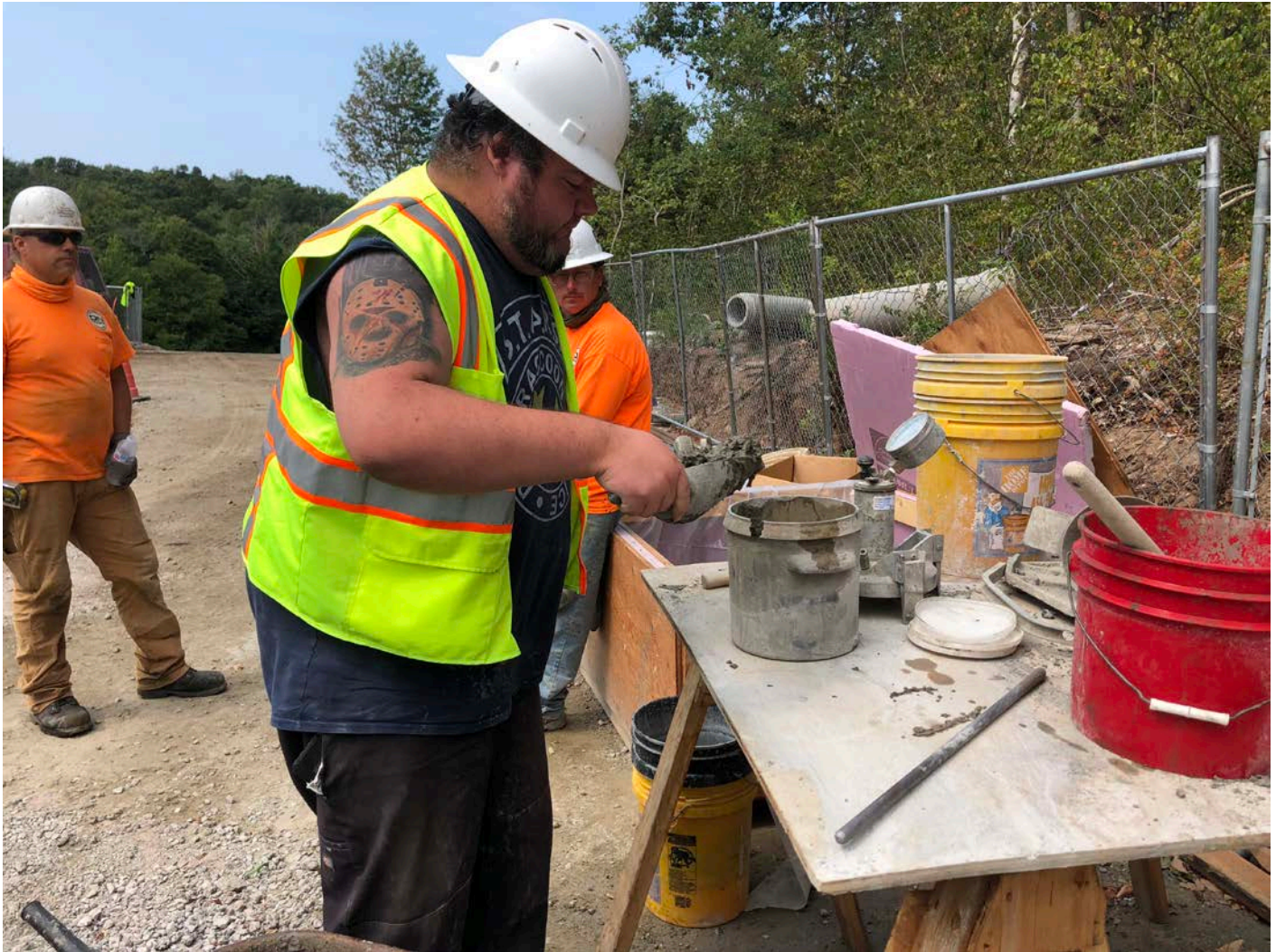
Picture 6: JTC collecting an air sample from the one truck of concrete brought to the water tank work zone today for placement on the water tank dome panels. Water tank work zone, east of the Shared Access Driveway, Middletown. View to the west.
