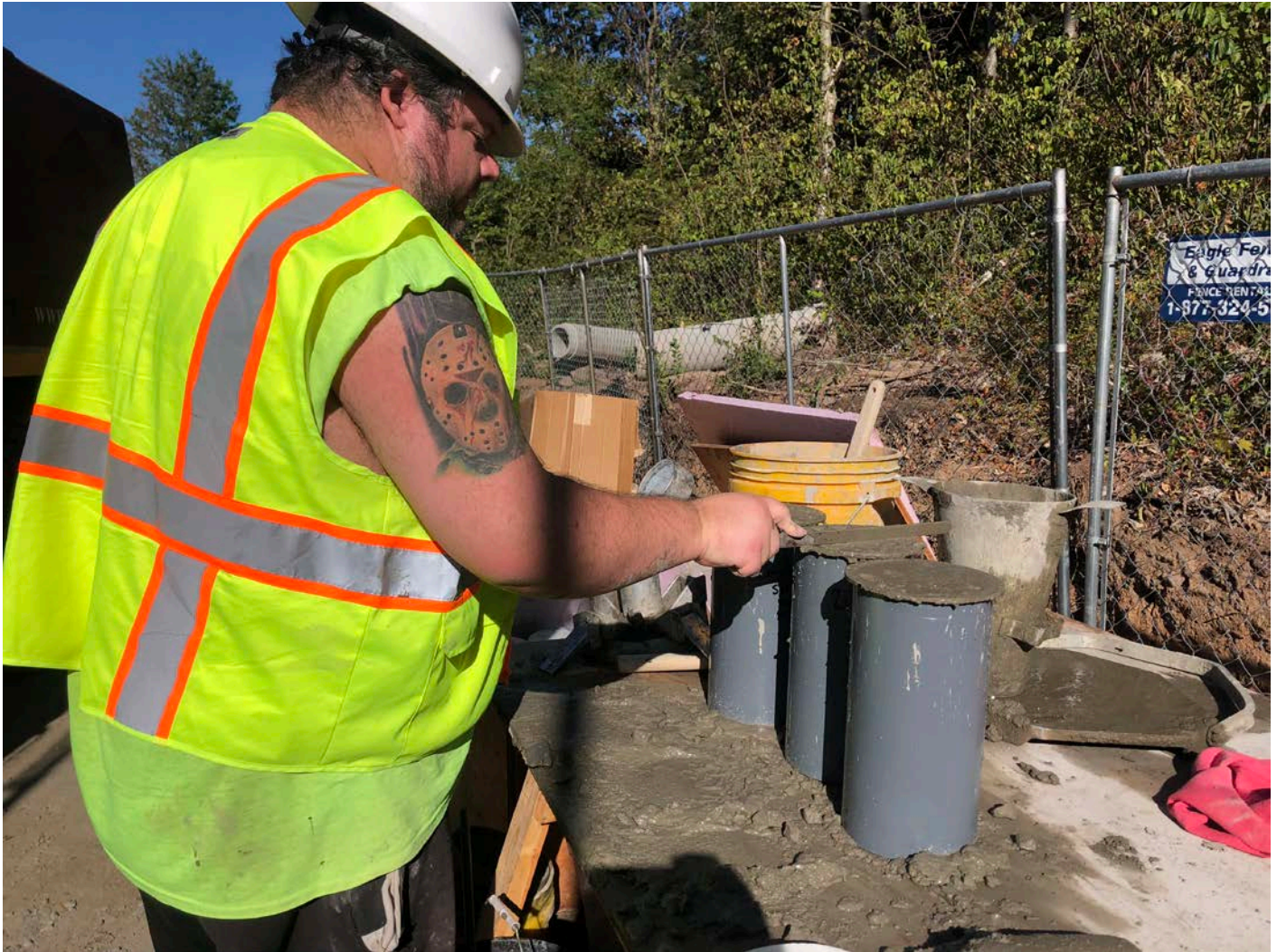
Picture 6: JTC collecting samples for laboratory analysis on concrete that was just delivered to the water tank work zone. Water tank work zone, east of the Shared Access Driveway, Middletown. View to the west.
