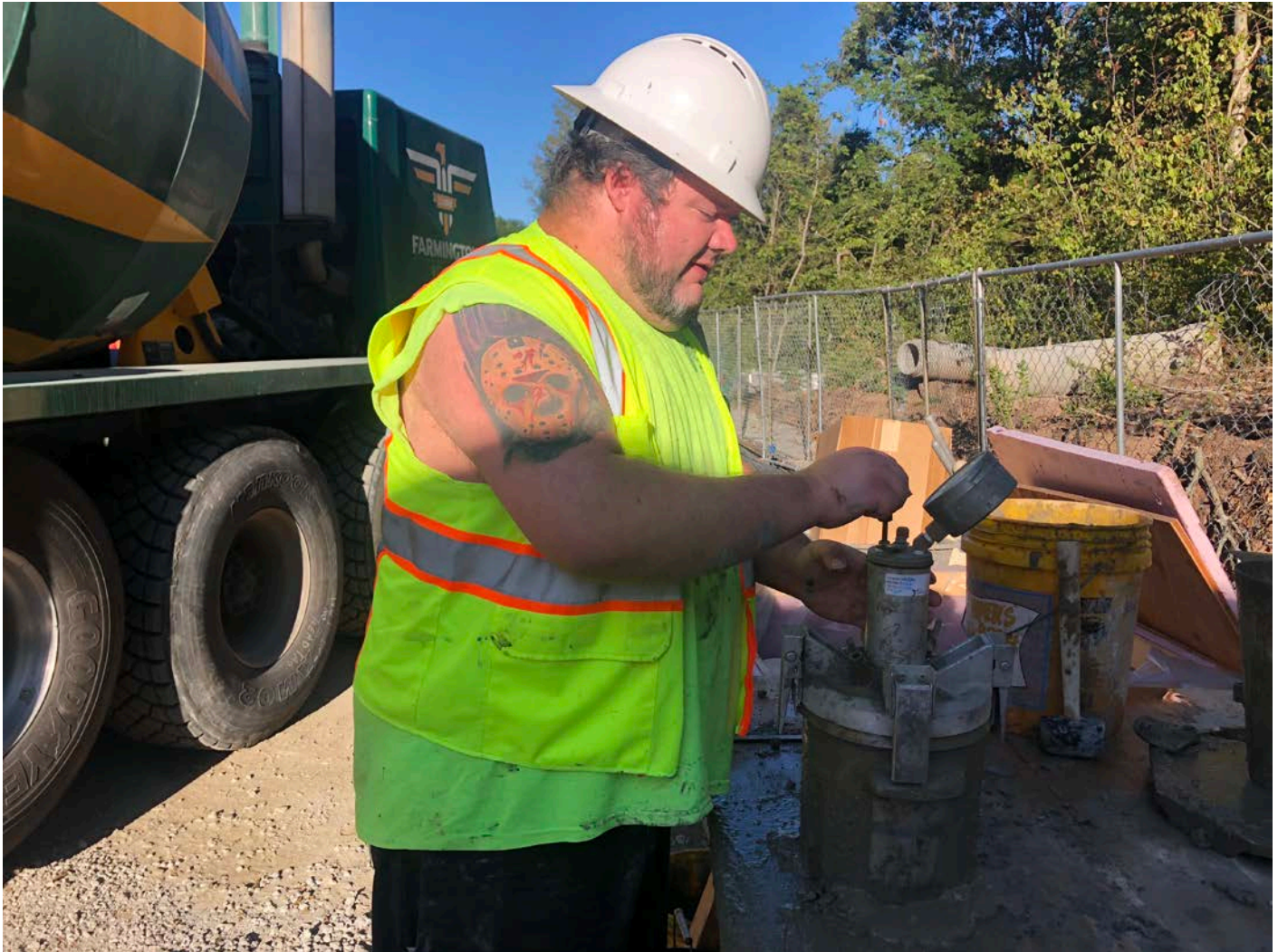
Picture 3: JTC performing percent air analysis on concrete that was just delivered to the water tank work zone. Water tank work zone, east of the Shared Access Driveway, Middletown. View to the west.
