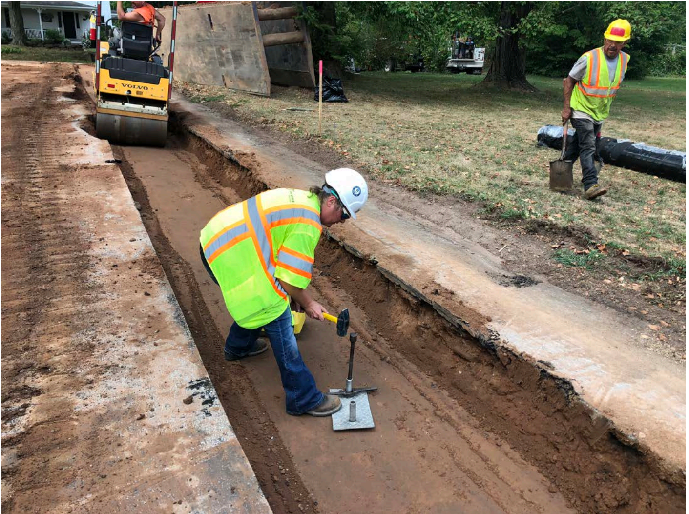
Picture 6: JTC performing soil compaction test on Talcott Lane, Durham. View to the west
