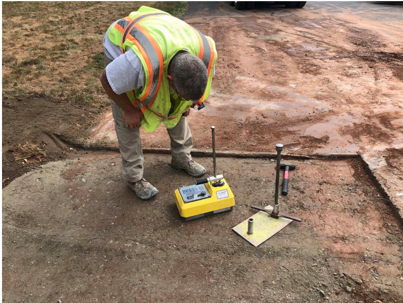
Picture 8: JTC collecting soil compaction data at the water service installation at 13 Maple Avenue, Durham. View to the north.
