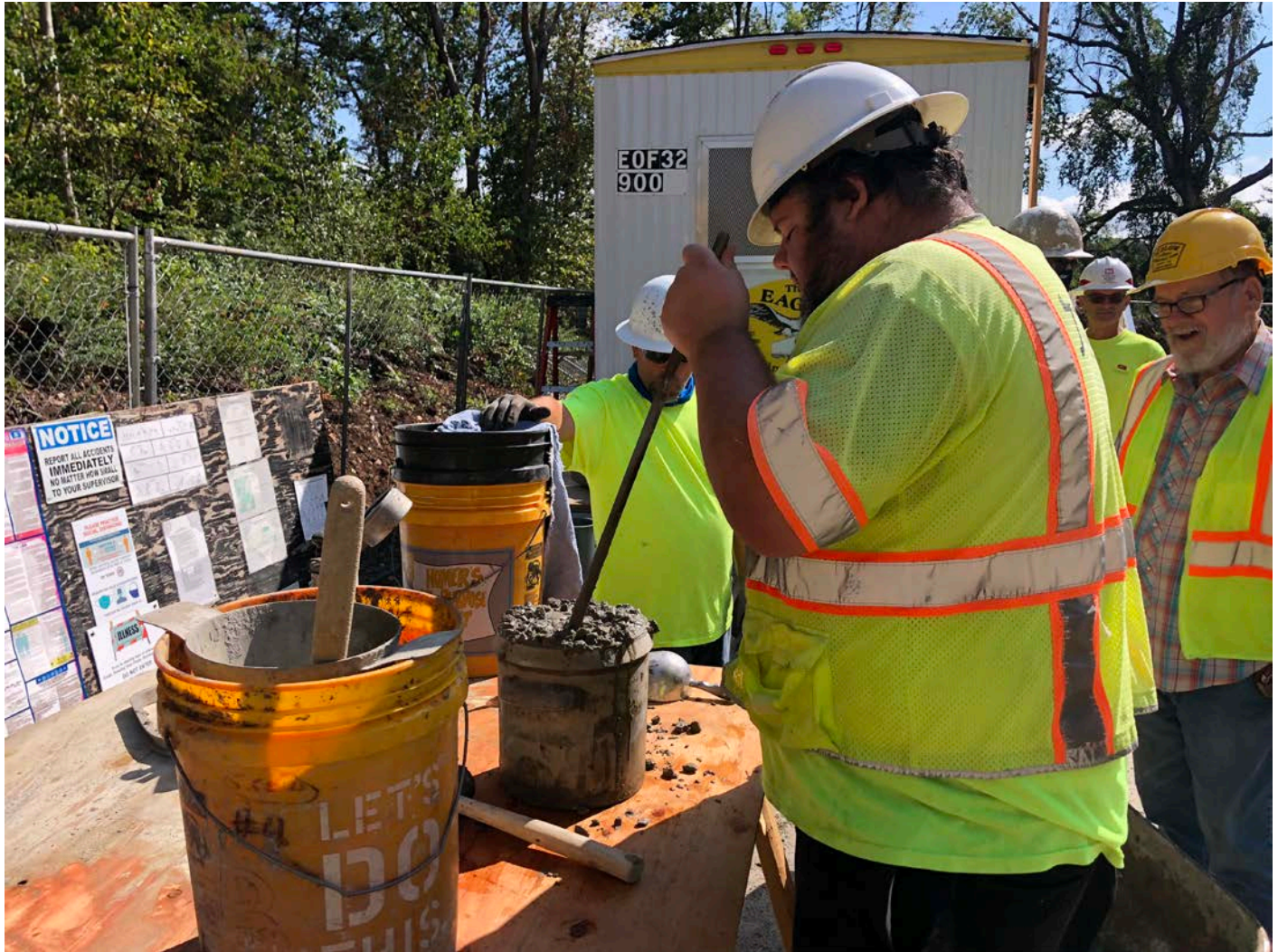
Picture 2: JTC preparing a concrete sample collected from the first of 6 concrete trucks to analyze for percent air. Water tank work zone, east of the Shared Access Driveway, Middletown.
